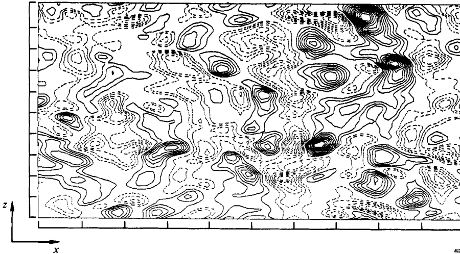
FIGURE 21. Contours of P in the (x, z) -plane at y^+ = 6.26 .
